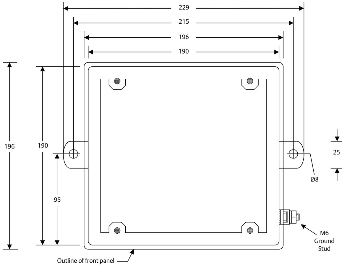
Overall depth = 100 mm (case and panel) + 3 mm (bracket) + 4.5 mm (bolt heads and washers)
