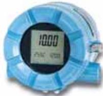
**The Model 56 Dual Input Analyzer** offers the choice of single or dual sensor inputs in any combination of pH/ORP, contacting or toroidal conductivity, chlorine, oxygen, or ozone. The analyzer features completely automatic air calibration for dissolved oxygen measurements.
