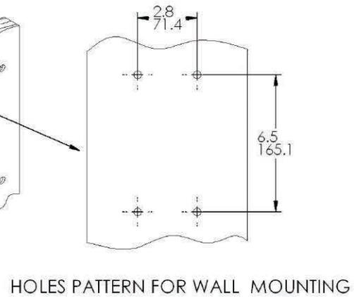
Wall Mounting Installation for 6081. Use Pipe/Wall Mounting Bracket Kit, PN 23820-00
