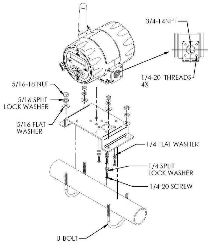
Pipe Mounting Installation for 6081. Use Pipe/Wall Mounting Bracket Kit, PN 23820-00
