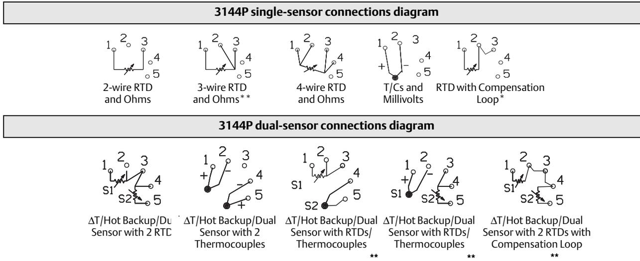
\* Transmitter must be configured for a 3-wire RTD in order to recognize an RTD with a compensation loop.
